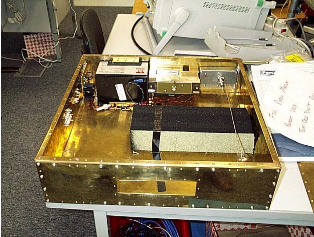
Figure 17: Representative EUT showing battery (top left), 7 GHz CNE (top centre), 2 GHz CNE (top right)
