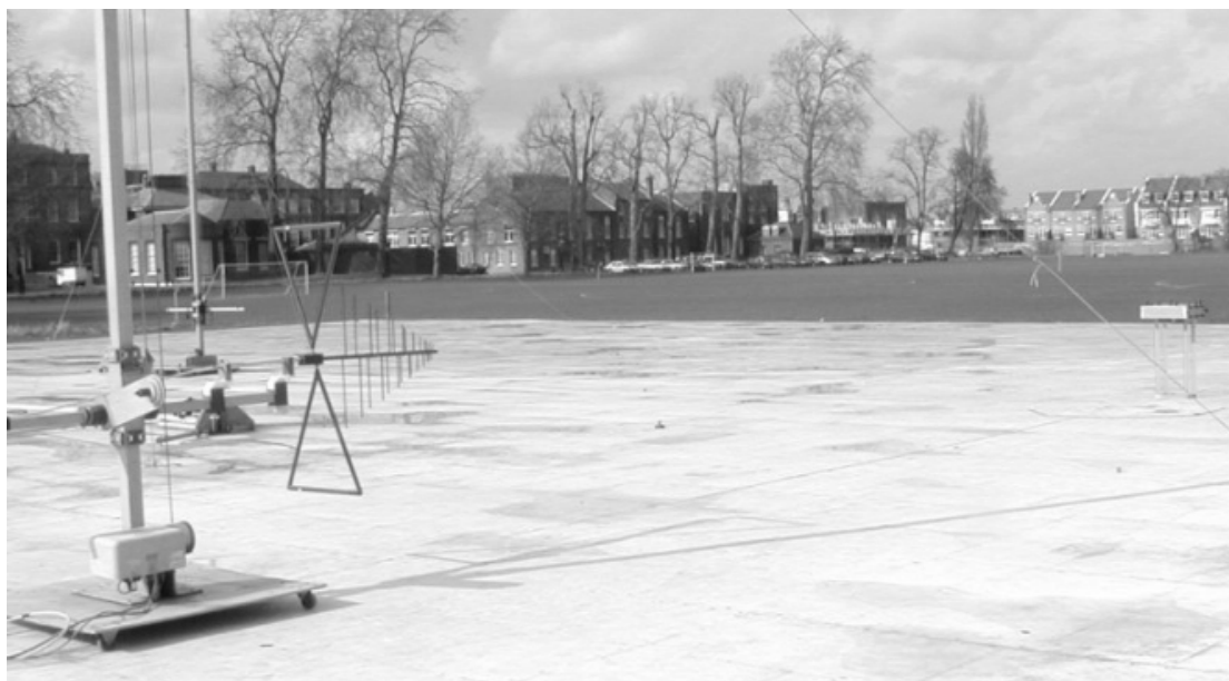
Figure 19: EUT measurement at 10 m range on short axis of NPL 60 m ground plane
