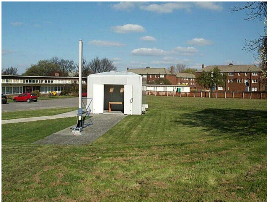
Figure 20: OATS at YES Castleford EMC Test Laboratory with the metallic ground plane, the mast and turning table.
