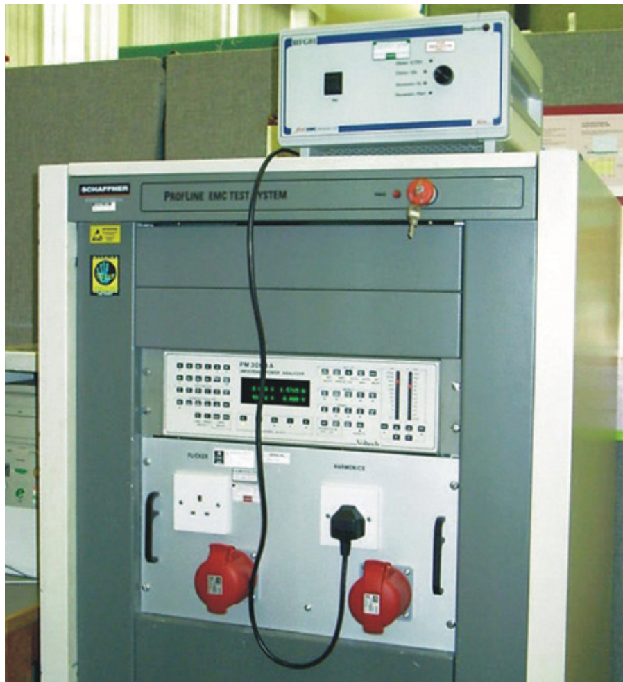
Figure 3. Harmonics pre-test using the HFG01 as the reference load
