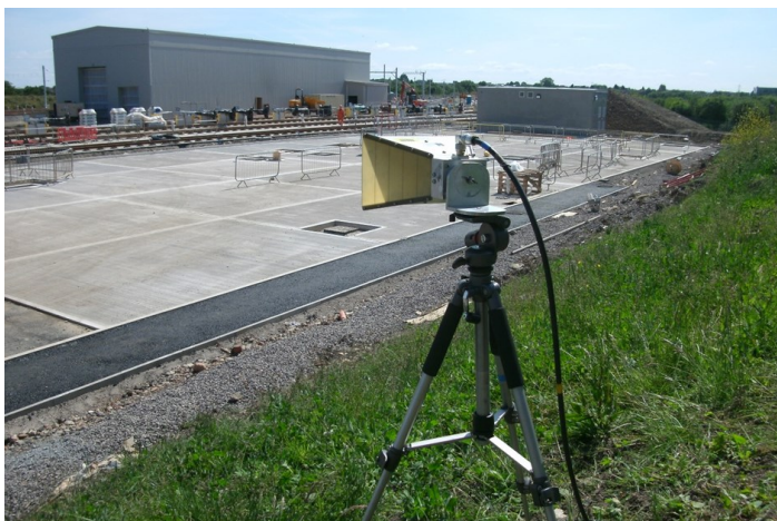
Figure 1: High frequency on-site EM measurements at a new-build Depot.
