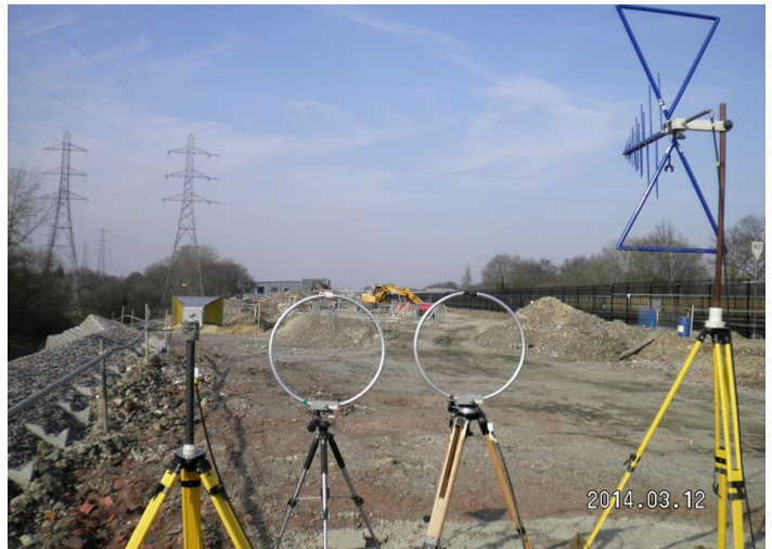
Figure 2: EM Site survey covering all frequency ranges being measured during construction of re-built depot.
