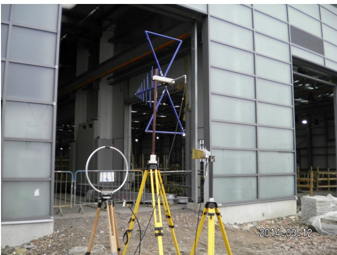
Figure 3: Measuring emissions at a location where the Risk Assessment suggests there will need to be a check once installation is complete.
